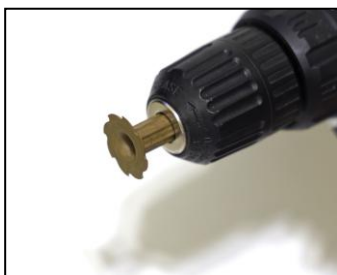
Attaching CSR to drill chuck interface
