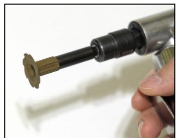
Attaching CSR with straight shank adapter
