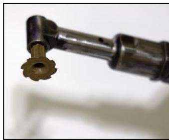
Attaching CSR to 1/4"-28 UNF interface
